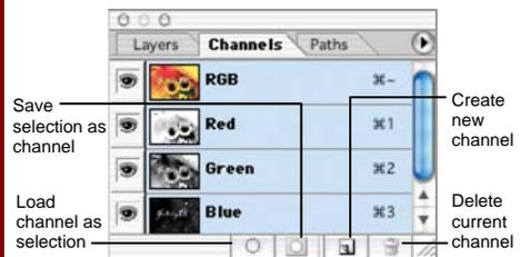
View individual color channels for the color model used in the image. The thumbnails appear in grayscale, but the image changes to display the selected channel(s).
