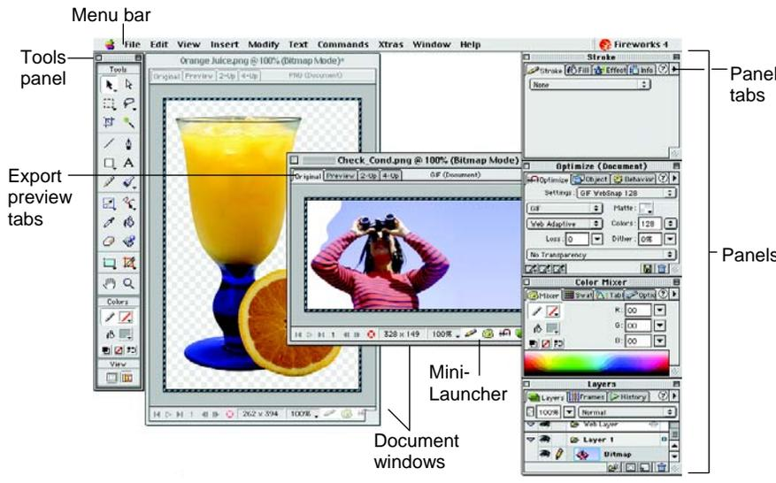
**To Display a Tool Group:** Click and hold down a tool with a small triangle in the lower-right corner of the button. Move the cursor to select another tool from the group. \*Use in bitmap mode. \*\*Use in vector mode.
